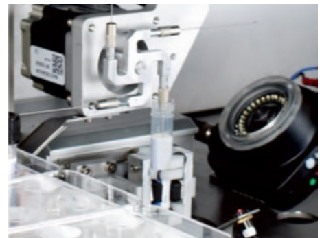
Figure 3. Onboard camera verifies sample is present on loop to ensure accurate sampling.
