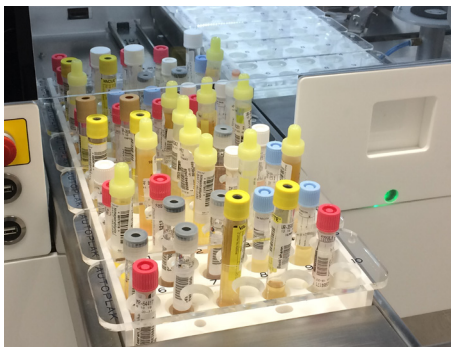
Figure 1. Universal rack allows multiple samples to be loaded randomly improving productivity and throughput.
